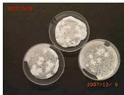
Figure 1. Melts in the process of crystallising from a glass form. The white areas are the crystalline polymer matrix. The samples are a triplicate.
